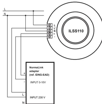
**Please note** Once the fitting is connected to mains and it is turned off, the relay will remain closed and the - + output will be at maximum while the stabilization takes place (approximately 1 minute).
