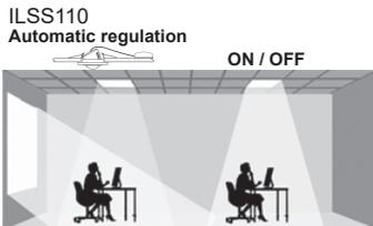
Install the sensor in the position to be taken as a luminosity reference (normally on top of the working space).
